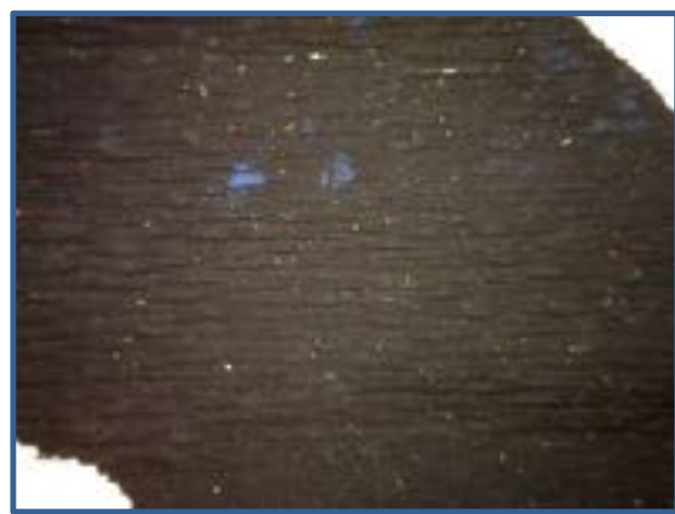
Image 2. Black paint displaying metallic pigments and other impurities. Taken at 20x magnification with transmitted light.
