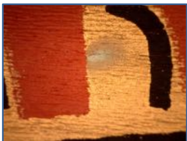
Image 1. Copper corrosion and hand-painted finishing details in black. Taken at 20x magnification with transmitted light.
