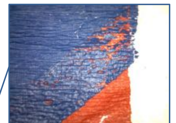
Image 5. Recto view. Overlap of blue and red paint. Taken at 20x magnification with transmitted light.
